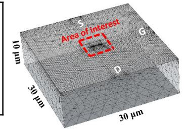
Fig. 11. Model design and mesh build-up of a TG In<sub>2</sub>O<sub>3</sub> device for thermal simulation with a finite-element method.
