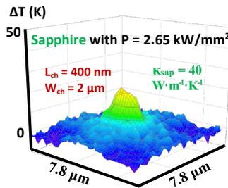
Fig. 8. Temperature increase of a TG In<sub>2</sub>O<sub>3</sub> transistor with sapphire substrate and power density of 2.65 kW/mm<sup>2</sup>.
