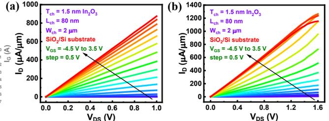
Fig. 3. Output characteristics of a TG In<sub>2</sub>O<sub>3</sub> transistor after O<sub>2</sub> annealing at 230 °C with  $L_{\text{ch}}$  of 80 nm, SiO<sub>2</sub>/Si substrate, and  $V_{\text{DS}}$  of (a) 1.0 V and (b) 1.6 V. The curves in (b) shows severe SHE at large  $V_{\text{DS}}$  with high  $I_{\text{D}}$ .
