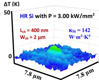
Fig. 9. Temperature increase of a TG In<sub>2</sub>O<sub>3</sub> transistor with HR Si substrate and power density of 3.00 kW/mm<sup>2</sup>.
