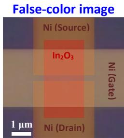
Fig. 12. A false-color image of a fabricated TG In<sub>2</sub>O<sub>3</sub> device with  $L_{\text{ch}}/W_{\text{ch}}$  of 0.4/2  $\mu\text{m}$ .
