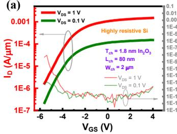
Fig. 18. (a) Transfer and (b) output characteristics of a TG In<sub>2</sub>O<sub>3</sub> transistor with  $T_{\text{ch}}$  of 1.8 nm,  $L_{\text{ch}}$  of 80 nm, and HR Si substrate after O<sub>2</sub> annealing at 235 °C achieving maximum  $I_{\text{D}}$  of 2.65 mA/ $\mu\text{m}$ .
