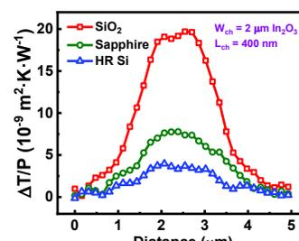
Fig. 10. Cross-sections of temperature increase of TG In<sub>2</sub>O<sub>3</sub> transistors with different substrates normalized by power density.
