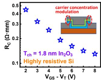
Fig. 17.  $R_{\text{c}}$  decreases with increasing  $V_{\text{GS}} - V_{\text{T}}$  due to carrier concentration modulation.
