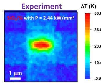
Fig. 14. TR measurement of a TG In<sub>2</sub>O<sub>3</sub> device with  $L_{\text{ch}}$  of 400 nm and  $W_{\text{ch}}$  of 2  $\mu\text{m}$ .
