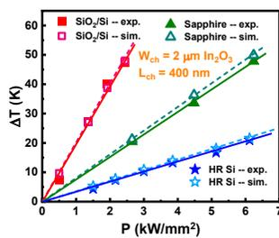
Fig. 16.  $\Delta T$  extraction of TG In<sub>2</sub>O<sub>3</sub> devices with different substrates and power density.
