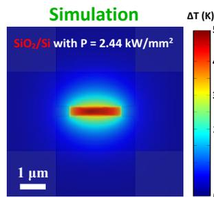
Fig. 13. Simulation result of a TG In<sub>2</sub>O<sub>3</sub> device with  $L_{\text{ch}}$  of 400 nm and  $W_{\text{ch}}$  of 2  $\mu\text{m}$ .
