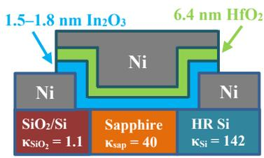
Fig. 1. Schematic diagram of TG In<sub>2</sub>O<sub>3</sub> transistors with different substrates. The unit of thermal conductivity ( $\kappa$ ) is  $\text{W}\cdot\text{m}^{-1}\cdot\text{K}^{-1}$ .
