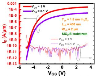
Fig. 2. Transfer characteristics of a TG In<sub>2</sub>O<sub>3</sub> transistor after O<sub>2</sub> annealing at 200 °C with  $L_{\text{ch}}$  of 400 nm, SiO<sub>2</sub>/Si substrate.
