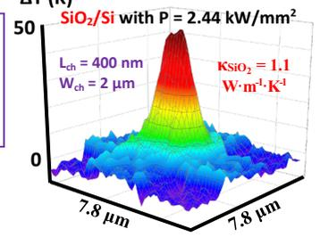
Fig. 7. Temperature increase of a TG In<sub>2</sub>O<sub>3</sub> transistor with SiO<sub>2</sub>/Si substrate and power density of 2.44 kW/mm<sup>2</sup>.
